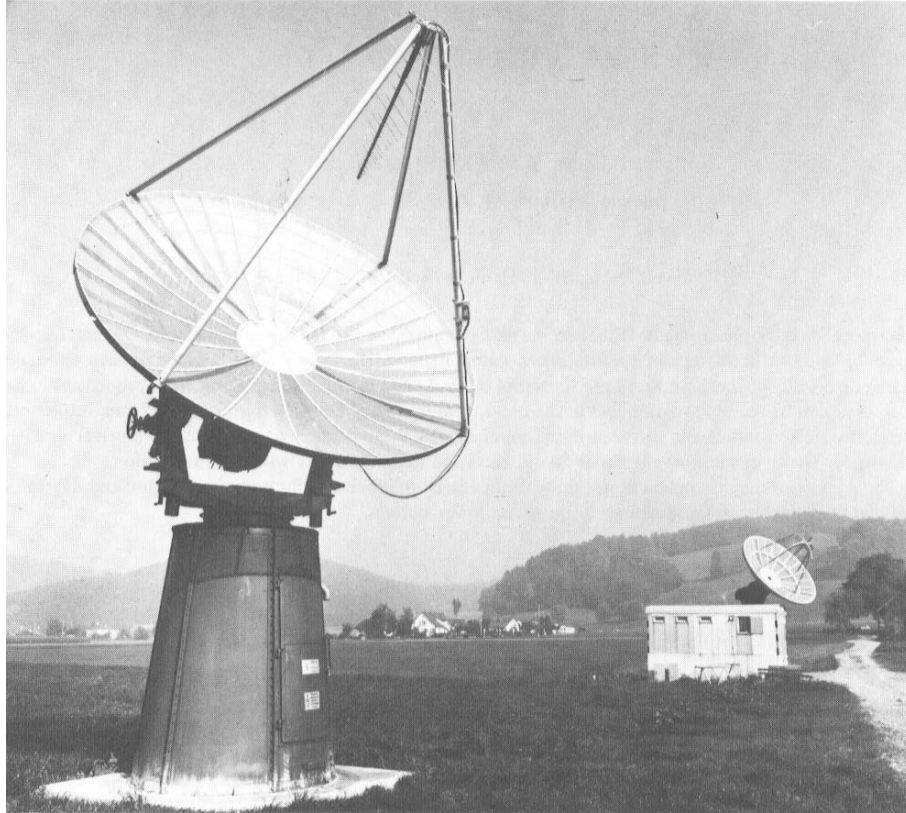
Figure 1: The radio observatory at Bleien. The 5 m „DAEDALUS“ dish is shown in the foreground. The 7 m „IKARUS“ dish is located behind the trailer with the computer and the receivers.
