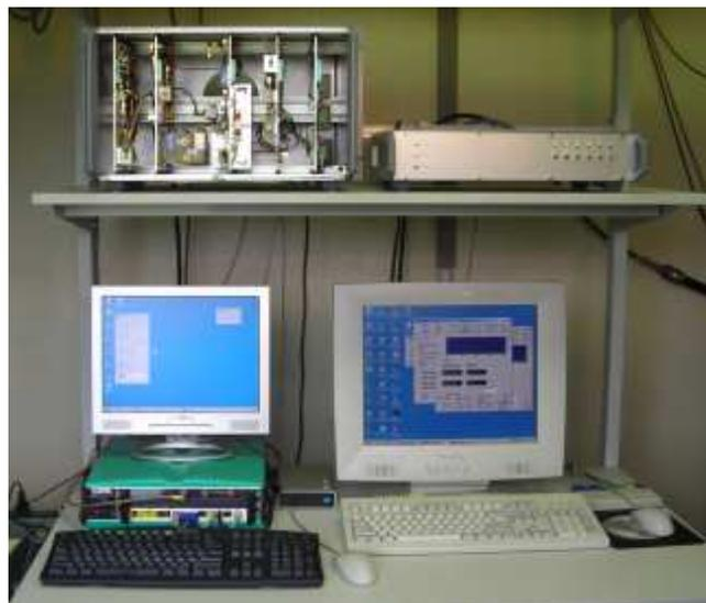
**Fig. 1.** Phoenix-3 receiver 1-5GHz for two polarizations top left, FPU-controller top right, FFT spectrometer ARGOS bottom left (green box) and FTP-server PERISCOPE bottom right at Bleien observatory, about 50 km south of Zurich.
